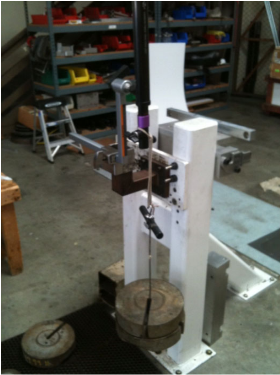
Figure 3. Custom TenZor carbon fiber orthopaedic traction unit undergoing calibration with weight stacks.
