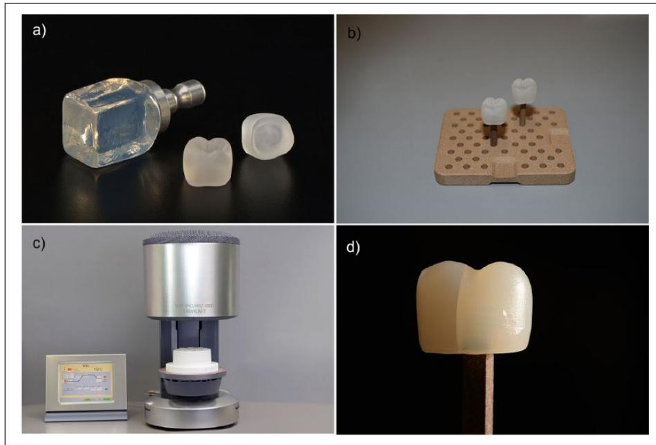
**Figure 1.** Lithium silicate material used for crown production (a), crowns on the firing pin (b), crystallization furnace with bottom-up lift system (c), and fractured crown after crystallization (d).
