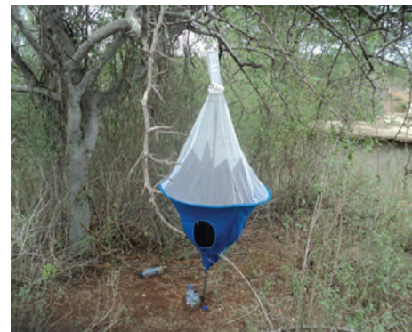
FIGURE 2: A biconical trap baited with cow urine and acetone to enhance trapping efficiency.
