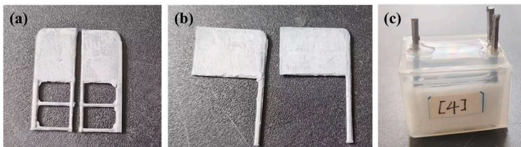
Fig. 1. Homemade simulated test battery.
