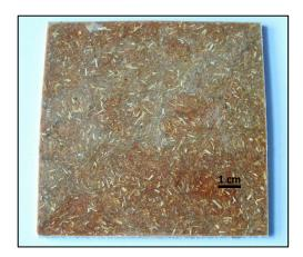
**Figure 1.** Chicken feather/PLA biocomposite containing 50 wt % of feather.
