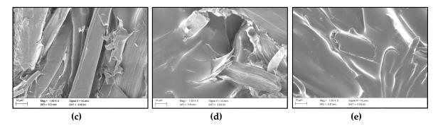
**Figure 9.** FE–SEM images of (**a**) untreated CFs; (**b**) NaOH-treated CFs; (**c**) fractured ING/CF (50/50); (**d**) fractured ING/NaOH–CF (50/50) and (**e**) fractured PEG–ING/CF (50/50).
