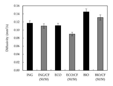
Figure 10. Diffusivity values of neat polymers and polymers reinforced with 50 wt % CFs.
