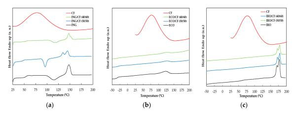
**Figure 5.** DSC curves of **(a)** ING-based biocomposites; **(b)** ECO-based biocomposites and **(c)** BIO-based biocomposites.
