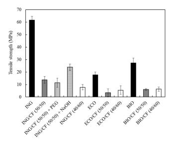
**Figure 7.** Tensile strength values of neat polymers and the different biocomposites containing 50 and 60 wt % of CFs.
