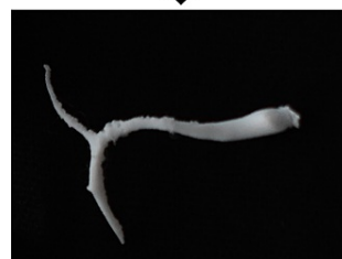
FIGURE 1: Fabricating the internal mold via 3D printing
