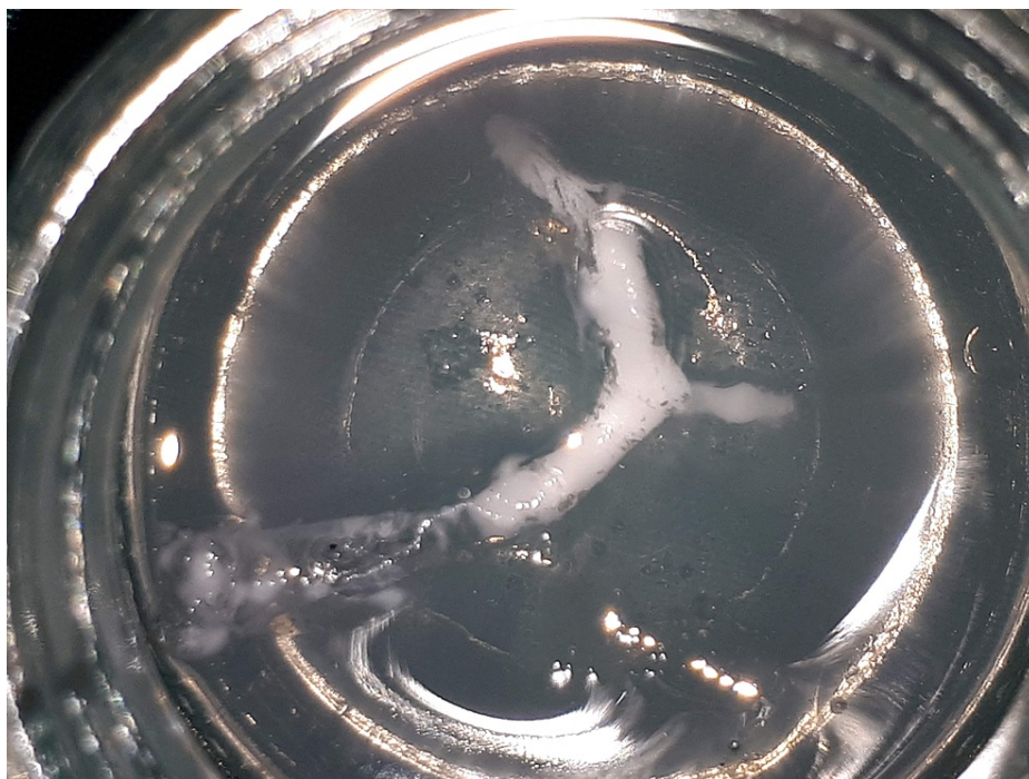
FIGURE 3: The model was placed in the chloroform bath until the internal mold dissolved
