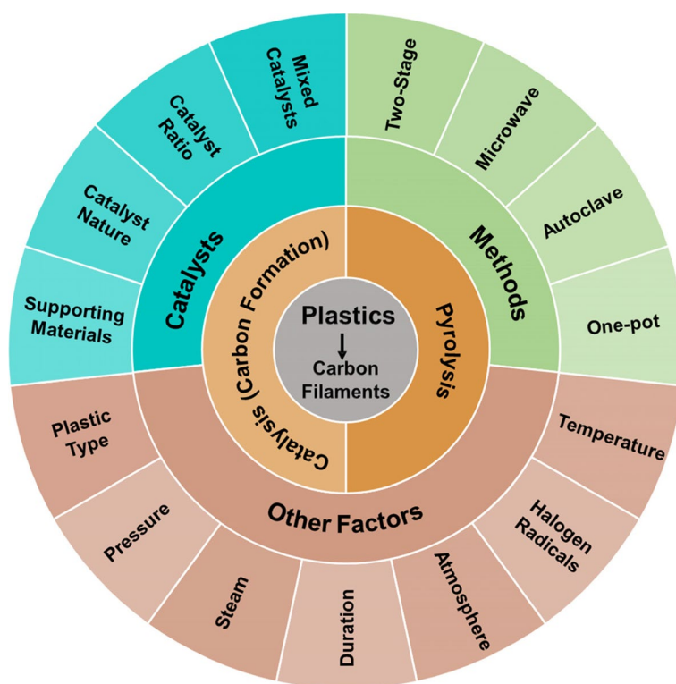
Fig. 2 The impact factors related to the conversion of plastics to carbon filaments
