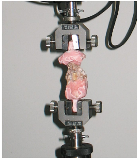
Figure 4. Biomechanical experimental setup for applying pure moments to the cervical segment. The sample was placed on a support jig mounted on the universal mechanical testing machine.
