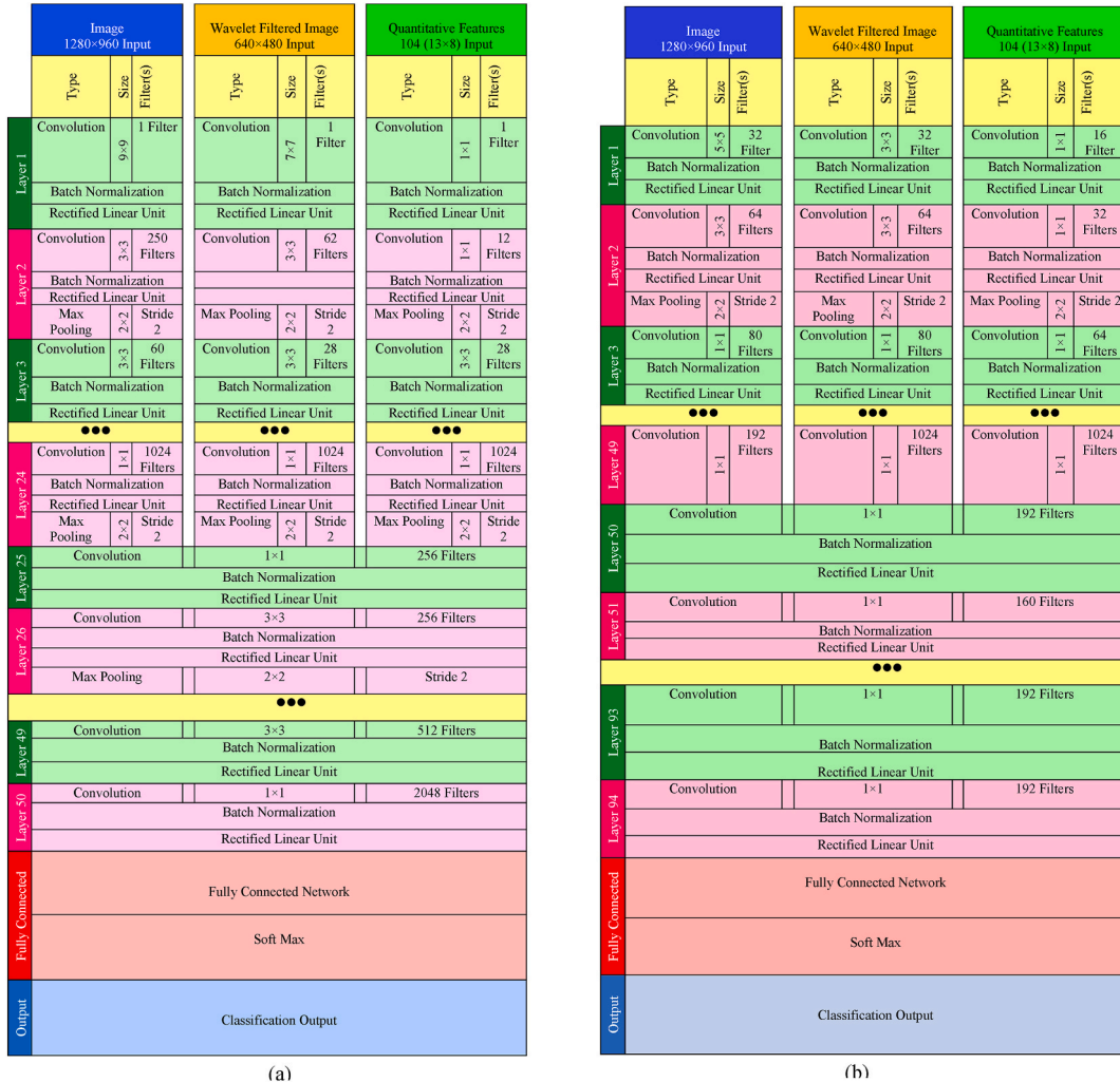
Fig. 5. The structure of (a) MP-ResNet-50 with 50 convolutional layers and (b) MP-Inception-V3 with 48 convolutional layers.
