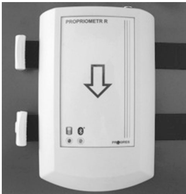
Fig. 2 X-panel of Propriometer—module of uniaxial transducer of the arm's position
