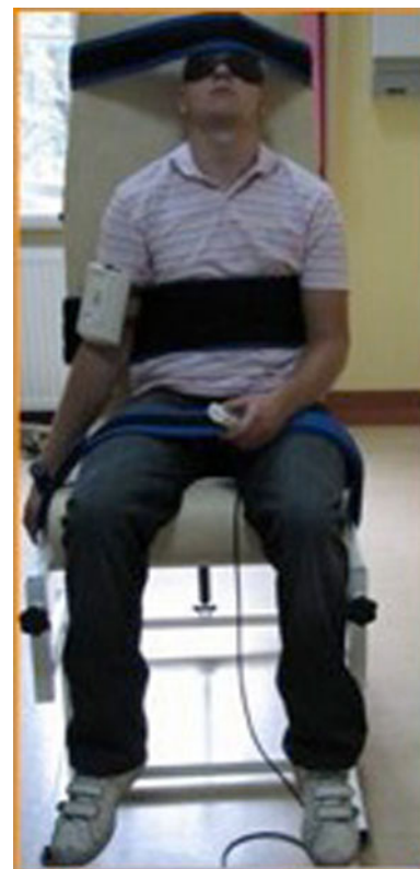
Fig. 4 Proprioception examination set-up: examinee's position for flexion and abduction position with assembled device
