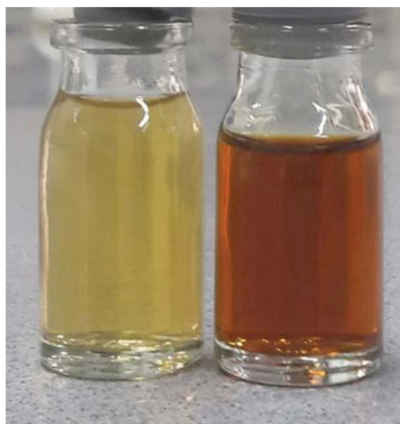
Fig. 1. The color change of plant extract (left) before and (right) after adding a silver nitrate solution
