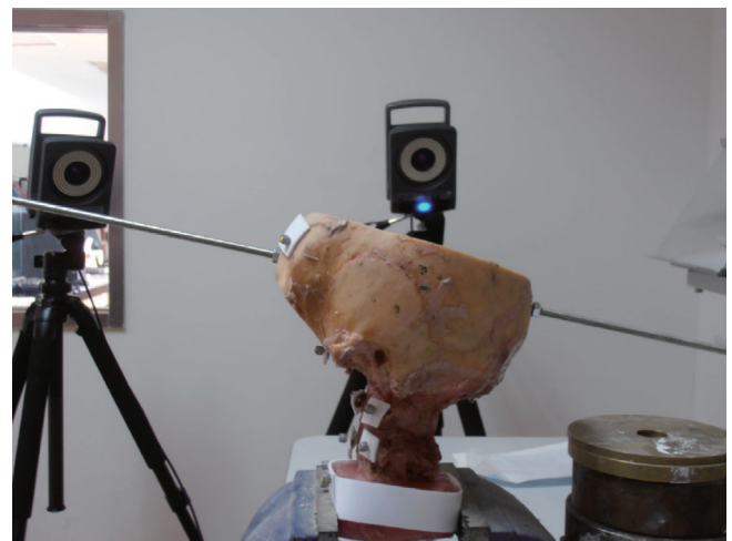
Fig. 3 ROM test. The prepared specimens were attached to the rigid base in a testing frame. Using a system of loading arms, pulleys, and weights, quasi-static loads were applied to the skull, leading to sequential pure moments of 0, 0.5, 1.0, 1.5, 1.0, 0.5, and 0 Nm. Moments were applied to generate the following 6 loading modes: extension; flexion; left and right lateral bending; and left and right axial rotation.
