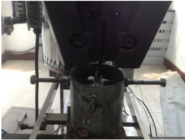
Fig. 4 Apparatus for testing pullout strength. A force was applied in line with the screw axis using a Servomotor at a rate of 0.25 mm/s. A force sensor was used to measure the tension at the cable.
