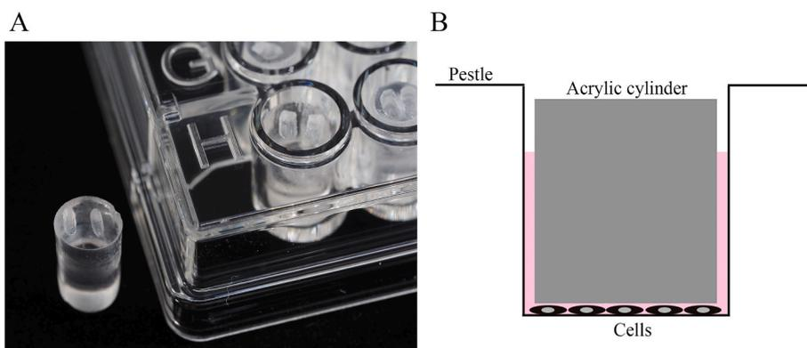
**Fig. 1.** Acrylic cylinders were laser-cut and placed into 96-well plates to apply compressive force. A: Photo of an acrylic cylinder; B: illustration of the hydrostatic pressure-generated compressive model.
