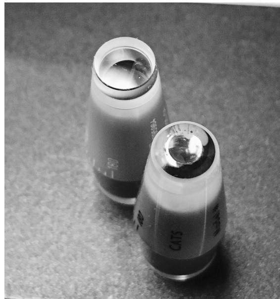
Figure 3 Photograph of the CATS tonometer prism and GAT prism applanating surfaces. Abbreviations: CATS, correcting applanation tonometry surface; GAT, Goldmann applanation tonometer.
