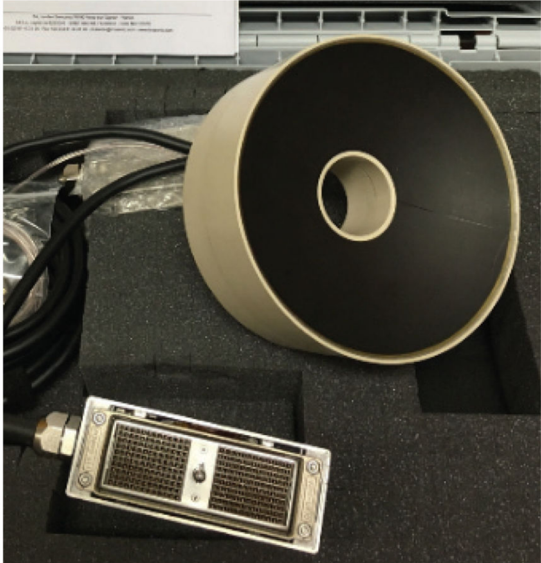
Fig. 6. Photo of the 256-element array transducer designed using the proposed method to generate shocks of 90 – 100 MPa at the focus. The final parameters of the array are: 1.5 MHz frequency, 144 mm aperture, 120 mm focal length ( F_{number} = 0.83 ), 256 elements of 7 mm diameter positioned with 0.5 mm gaps in 16–arm spiral configuration, and 40 mm central opening for a P4-2 ultrasound imaging probe.
