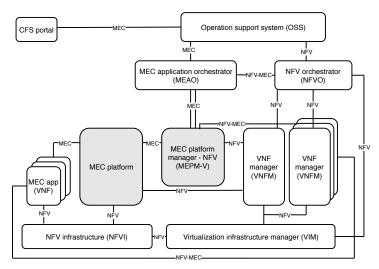
Figure 2. ETSI NFV MEC architectural framework.
