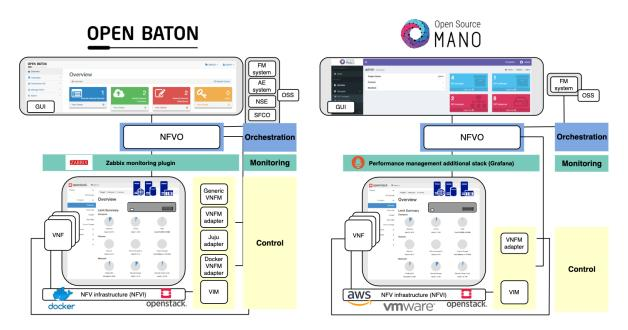
Figure 6. Open Baton and OSM architectures mapped to ETSI NFV MANO.
