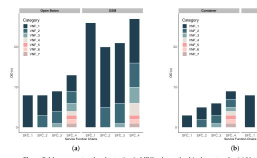
**Figure 7.** Management and orchestration in MEC-enhanced vehicular networks. (a) Network service instantiation delay: Open Baton vs. OSM. (b) Network service instantiation delay: Docker Containers vs. VMs.
