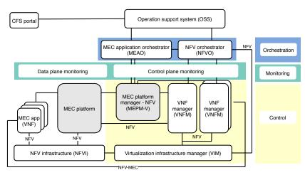
**Figure 3.** The closed-loop life-cycle managment of network services mapped to ETSI NFV MEC architectural framework.
