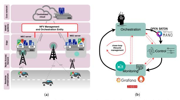
**Figure 1.** Management and orchestration in MEC-enhanced vehicular networks. (a) A high-level architecture of MEC-enhanced vehicular networks. (b) The closed-loop life-cycle management of network services.
