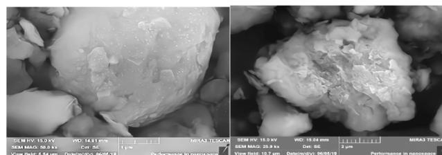
**Figure 10.** SEM images before and after dissolution of cuttings.
