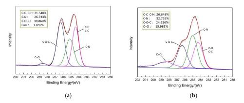
Figure 13. Component-fitted XPS spectra of the C1s peaks of polyurea coating (a) before and (b) after aging.
