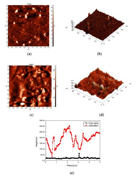
**Figure 9.** AFM of polyurea coating (**a**) 2D topographic image of PCB; (**b**) 3D topographic image of PCB; (**c**) 2D topographic image of PCA; (**d**) 3D topographic image of PCA; and (**e**) the height of surface before and after 150 d aging.
