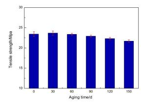
Figure 5. Tensile strength of polyurea coating.
