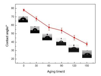
Figure 4. Change in contact angle with aging time.
