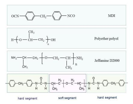
Figure 1. Molecular structures of polyurea precursors.
