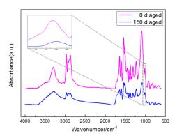
**Figure 11.** FTIR spectra at the region of 4000–500 cm<sup>-1</sup> for unaged and aged polyurea.
