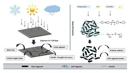
Scheme 1. Schematic illustration of the aging mechanism of polyurea coating.
