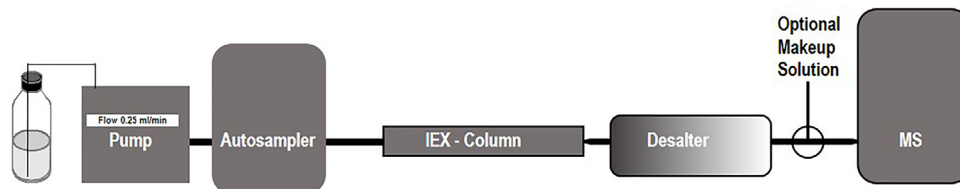
FIGURE 1 Instrumental setup of ion chromatography coupled to mass spectrometry
