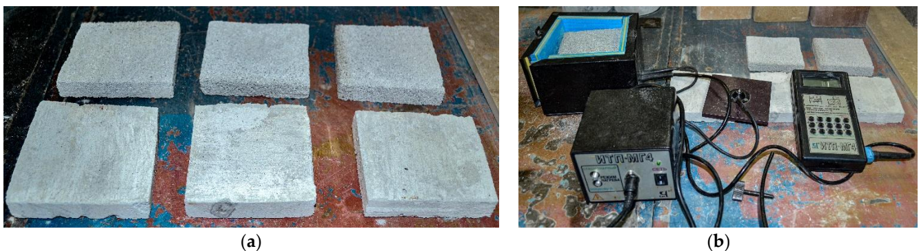
Figure 2. Specimens (a) and device (b) for testing aerated concrete for thermal conductivity.
