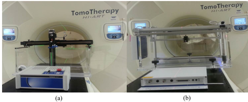
FIG. 1. Schematic of the hardware setup for two water scanning systems in the tomotherapy (TOMO) machine: (a) Standard Imaging TomoScanner (TS) and (b) IBA Blue Phantom Helix (BPH).
