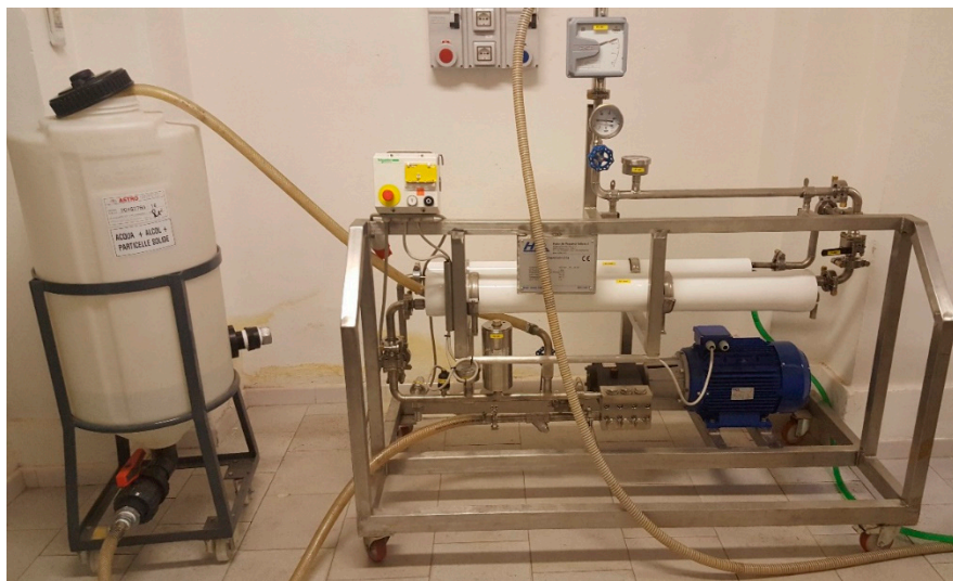
Figure 7. Hydro Air Research Italia pilot unit for ultra-, micro-, and nano-filtration ('green technologies development platform', DSTF, University of Turin, Turin, Italy).
