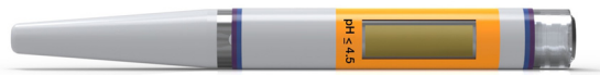
Figure 1 The RightSpotpH™ indicator device connects to a standard nasogastric tube, allowing aspiration of fluid into a chamber containing pH-indicating paper that changes color for pH < 4.5.
