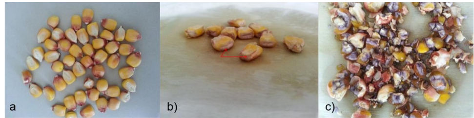
Fig 1. a) Waxy maize grain before iodine test; b) Brownish coloration in endosperm after iodine test; c) Formation of blue-purple color after iodine application in normal maize divided grains.
