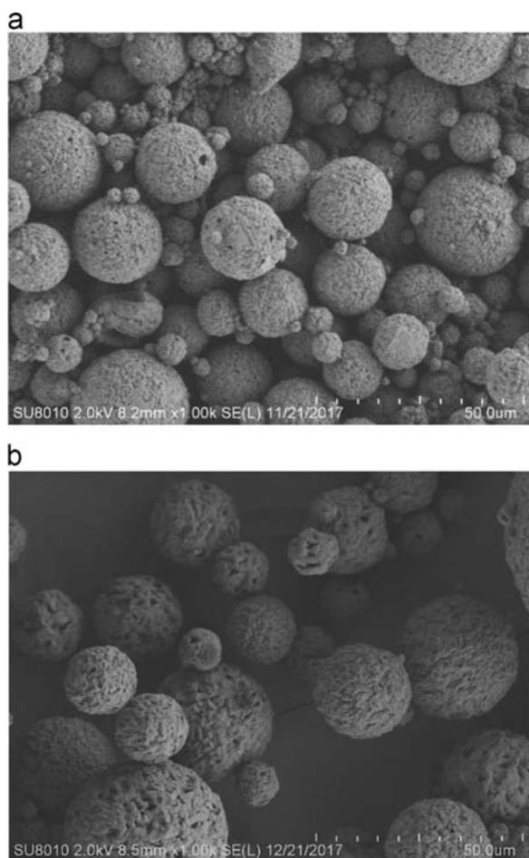
**Fig. 1.** Scanning electron microscopy (SEM) of produced PHA-based microbeads. (a) SEM of homopolymer, P(3HB) microbeads with 1000  $\times$  magnification. (b) SEM of copolymer, P(3HB-co-3HV) microbeads with 1000  $\times$  magnification.
