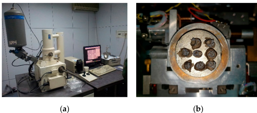
Figure 4. ZEISS LEO-1430 VP SEM system. (a) Scanning system; (b) Test samples coated with conductive film.
