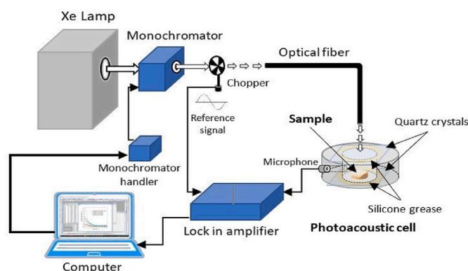
Fig. 2. Scheme of PAS experimental setup used in our experiments.
