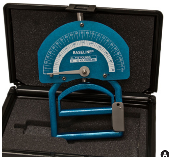
Fig. 3. Mechanical type dynamometer (Smedley type). (A) Baseline. (B) Takei, GRIP-A.
