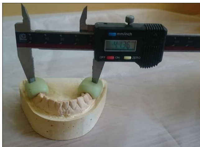
Figure 3: Measuring the distance between the two indexes by a standard digital caliper
