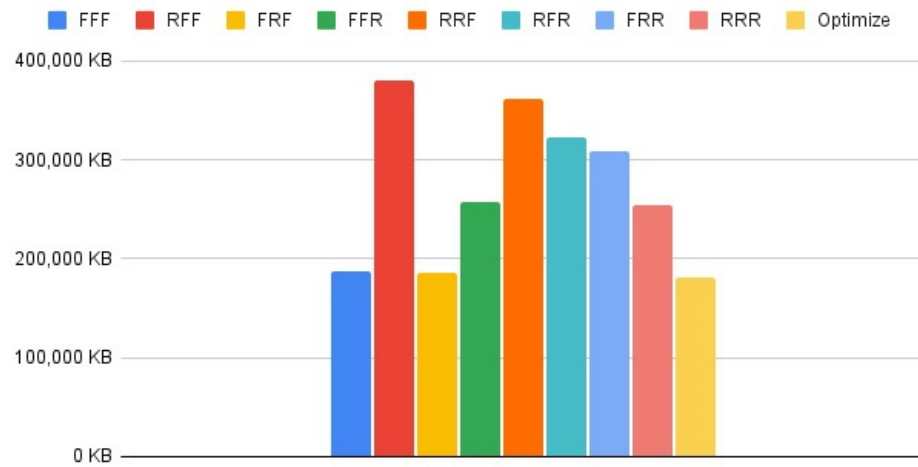
Figure 14. Total DRAM access—HarDNet39 (1024 PE/128 KB Buffer).
