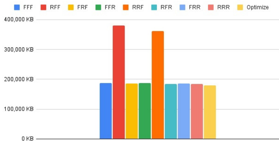
Figure 12. Total DRAM access—HarDNet39 (1024 PE/256 KB Buffer).
