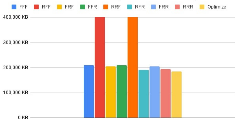
Figure 13. Total DRAM access—HarDNet39 (256 PE/256 KB Buffer).
