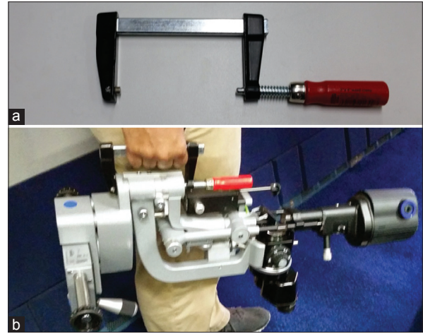
Figure 7: (a) "Four inch clamp" used to hold the slit lamp, (b) slit lamp being carried using the clamp
