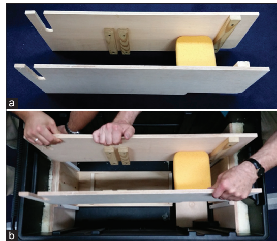
Figure 3: (a) Central unit on which the slit lamp would lay down, (b) central unit after being fitted into the toolbox
