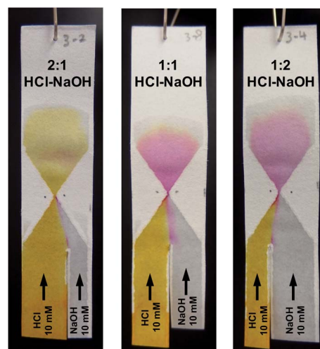
Fig. 6 The effect of varying the reagent channel width ratio on the composition of the mixture. The left reagent channel was suspended in 10 mM HCl solution, containing 2 mM of Phenol Red. The right reagent channel was suspended in a 10 mM NaOH solution. The width of these reagent channels was varied in order to change the composition of the mixture beyond the hourglass structure. As the contributions of each solution vary, so does the final pH of the mixture, as evidenced by the different colours exhibited by the Phenol Red, a pH-sensitive dye. Essentially, the gap widths of these hourglass structures are <0.5 mm. The HCl and NaOH channel widths for 2 : 1, 1 : 1 and 1 : 2 are approx. 10 and 5 mm; 8 and 8 mm; and 5 and 10 mm, respectively.
