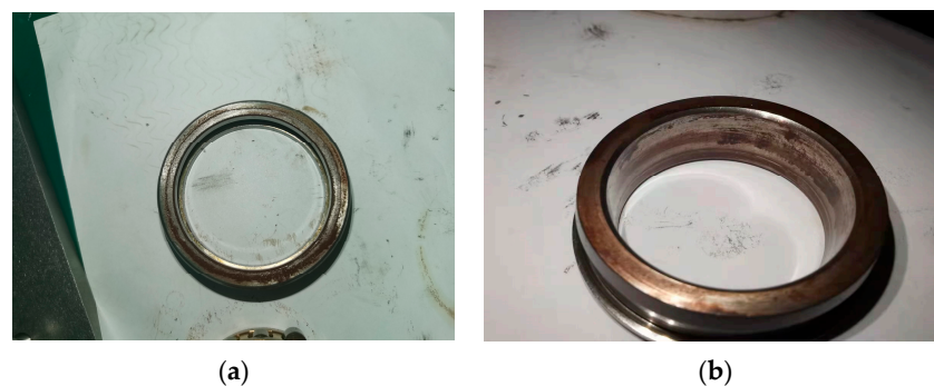
Figure 15. Partial diagram of experimental bearing failure: (a) outer ring failure; (b) inner ring failure.
