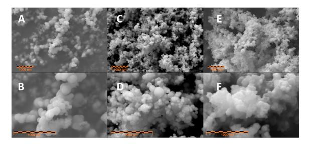
**Figure 2.** SEM images of pristine Si NPs (**A**,**B**), Si-1 (**C**,**D**) and Si-2 (**E**,**F**) samples. Upper figures—magnification 20,000×, lower—50,000×.
