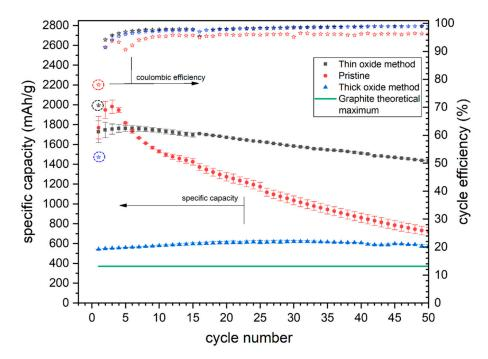
**Figure 6.** Pristine (red), Si-1 (black) and Si-2 (blue) galvanostatic charge/discharge results. Stars—coulombic efficiency. Squares, circles and triangles—specific delithiation capacities. Green line—theoretical capacity of graphite (372 mAh/g).
