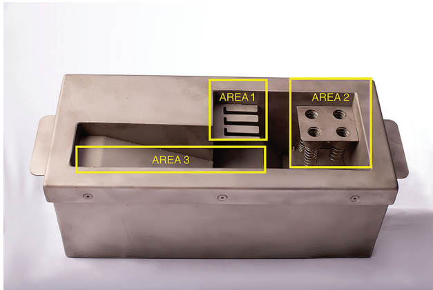
Figure 3. Vitrification equipment. Area 1: vitrification of oocytes and embryos; Area 2) lodging of cryotubes for the vitrification of germinative tissue; and Area 3) vitrification ramp.
