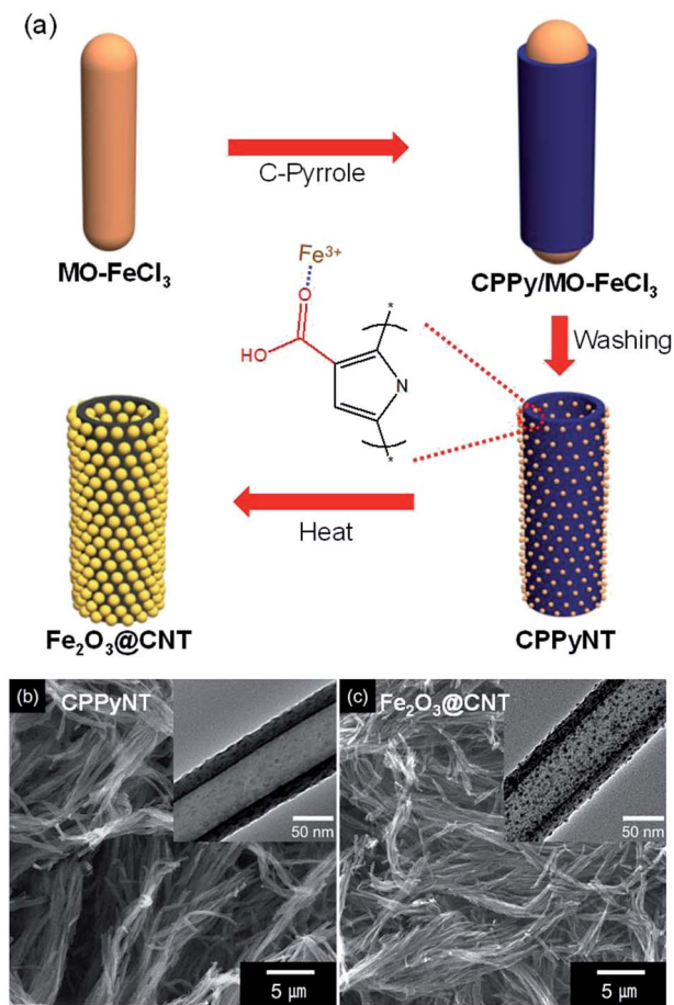
Fig. 1 (a) Illustrative of the sequential synthesis of the iron oxide decorated carbon nanotube composites. Field-emission scanning electron microscopy (FE-SEM) and transmission electron microscopy (TEM) (inset) images of (b) the carboxylated polypyrrole nanotubes (CPPyNT) and (c) the iron oxide decorated carbon nanotubes ( \text{Fe}_2\text{O}_3@CNT ).
