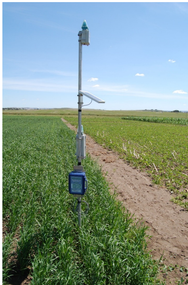
Figure 1. Watermark sensors (IRROmesh) wireless assembly in barley plots at the Nesson location.
