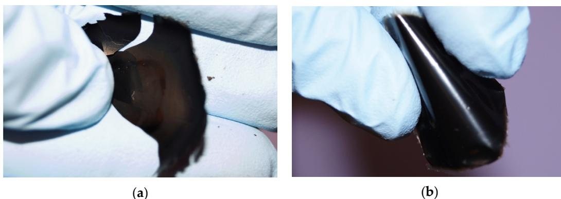
**Figure 2.** Cross-linked PPy–Alg films prepared from composite A (a) without and (b) with NaCO<sub>3</sub>.
