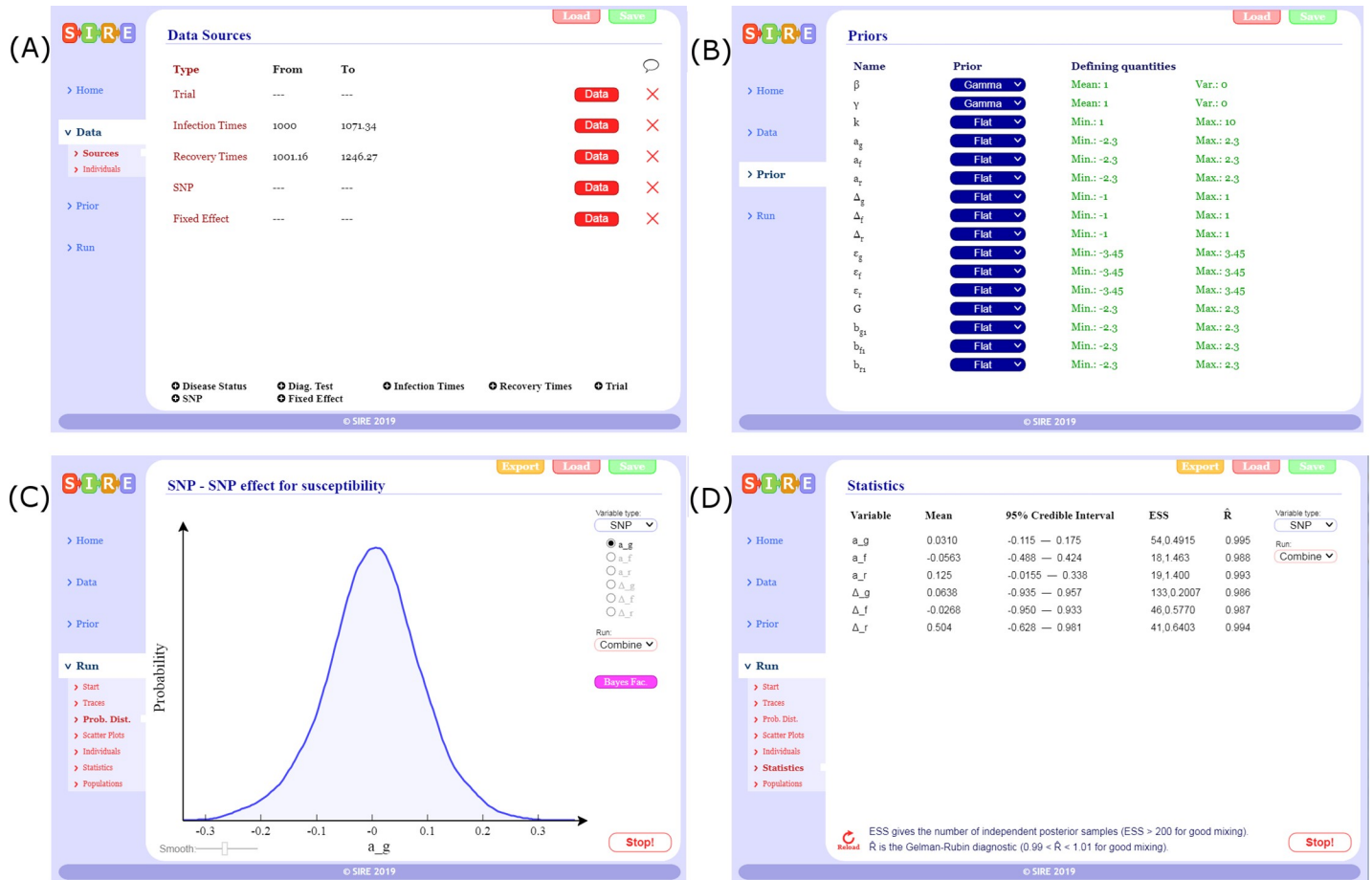
Fig 1. SIRE software. Illustrative screenshots of the software package: (A) Different data sources can be imported by loading user defined data tables (text or csv files), (B) prior specification can be made on parameters, (C) posterior distributions can be visualised as inference is being performed, and (D) summary statistics and MCMC diagnostics.
