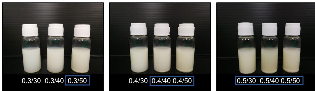
**FIGURE 3** GOZNs emulsions prepared using different zein concentration/ % GO loading, stored for 24 hr at 25°C. Precipitation in the square could be observed
