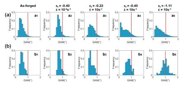
**Figure 11.** GAM histogram plots derived from EBSD data for: (**a**) all grains and (**b**) sheared coarse grains as the cyan group under varied conditions including the as-forged state, deformed states with  $\varepsilon_t$  of -0.22 at  $10^{-3}$  s<sup>-1</sup> and with  $\varepsilon_t$  of -0.22, -0.40 and -1.11 at 10 s<sup>-1</sup>.
