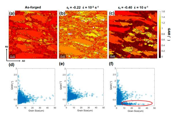
**Figure 7.** GAM maps for the microstructures in: (**a**) the as-forged state, deformed state with  $\varepsilon_t$  of -0.40 (**b**) at  $\dot{\varepsilon}$  of 10 s<sup>-1</sup> and (**c**) at  $\dot{\varepsilon}$  of  $10^{-3}$  s<sup>-1</sup>. The corresponding plots of grain size versus the GAM value are plotted in (**d**–**f**). The yellow ellipse in (**f**) highlights the occurrence of grown equiaxed grains with low GAM value and large grain size.
