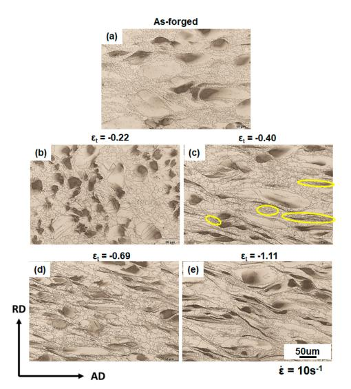
**Figure 4.** Optical micrograph of microstructures after compression with  $\varepsilon_t$  of (**a**) 0, (**b**) -0.22, (**c**) -0.40 (**d**) -0.69, and (**e**) -1.11 at 350 °C and 10 s<sup>-1</sup>. Yellow ellipses highlight refined DRXed grains formed near the Zr-rich coarse grains.
