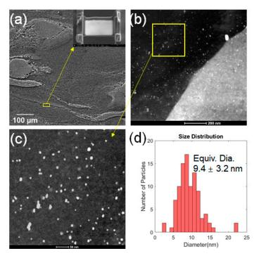
**Figure 14.** (a) SEM image of the selected area for FIB life-out membrane from the sample deformed to  $\varepsilon_t$  of -0.40 at  $\dot{\varepsilon}$  of  $10 \text{ s}^{-1}$ , (b) HAADF image in STEM mode for the sample lifted out in (a), (c) nano-sized Zn–Zr particles, and (d) size distribution histogram quantified from the micrograph in (c) showing the mean equivalent diameter of these Zn–Zr particles was about 9.4 nm.
