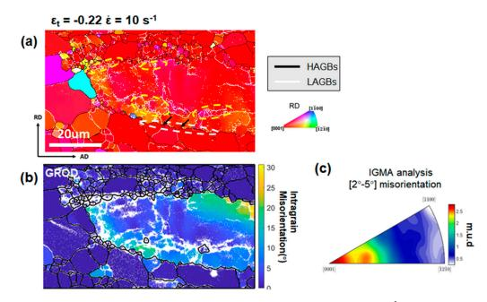
**Figure 12.** (a) IPF map of the microstructure deformed to  $\varepsilon_t$  of -0.22 at  $\dot{\varepsilon}$  of  $10 \text{ s}^{-1}$  with a step size of 0.12 µm, with sub-grains marked by yellow ellipses, serrated boundaries marked by a white ellipse, and refined DRXed grains marked by black arrows. (b) GROD map calculated from (a), and (c) IGMA analysis of the coarse grain shown in (b).
