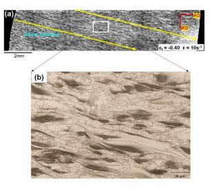
**Figure 3.** Optical micrographs of macro-SBs at  $\varepsilon_t$  of -0.40 under the high-strain-rate condition: (a) overall microstructure at a lower magnification, (b) microstructure in the framed region of (a) at a higher magnification.
