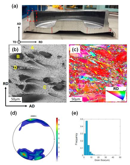
**Figure 1.** Initial microstructure of the as-received sample: (**a**) location of sampling for hot compression, (**b**,**c**) corresponding optical microscope (OM) and electron back-scattered diffraction (EBSD) micrographs of (**a**), (**d**) corresponding (0001) pole figure, and (**e**) grain size distribution calculated from the EBSD dataset of (**c**). The step size for EBSD measurements was 0.3 μm.
