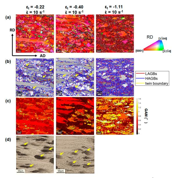
**Figure 6.** EBSD characterization of the microstructures deformed to  $\varepsilon_t$  of -0.22, -0.40, -1.11 at  $10 \text{ s}^{-1}$ : (a) IPF maps and (b) GBC maps superimposed by grain boundaries, (c) GAM maps and (d) corresponding optical micrographs for the same ROIs. The step size for EBSD measurements was  $0.3 \mu m$ . Yellow arrows indicate that dark-grey contrasted region in (b) correspond to Zr-rich domains in (d).
