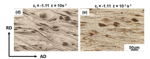
**Figure 5.** Optical micrographs of microstructures in different states: (**a**) as-forged state, after deformation at  $\dot{\epsilon}$  of 10 s<sup>-1</sup> with  $\epsilon_t$  of (**b**) -0.40 and (**d**) -1.11, after deformation at  $\dot{\epsilon}$  of 10<sup>-3</sup> s<sup>-1</sup> with  $\epsilon_t$  of (**c**) -0.40 and (**d**) -1.11.
