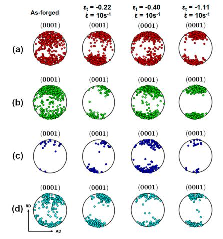
**Figure 10.** {0001} pole figures of four groups of grains: (**a**) Zr-rich refined grains as the red group, (**b**) Zr-lean refined grains as the green group, (**c**) Zr-lean grown equiaxed grains as the blue group and (**d**) sheared coarse grains as the cyan group.
