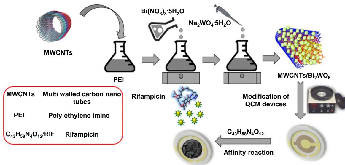
Figure 6. Scheme for fabricating a quartz crystal microbalance (QCM)-based rifampicin sensor using multiwalled carbon nanotubes (MWCNT) and Bi 2 WO 6 [90].
