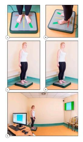
**Figure 1.** Stability measurement on a stable platform: (**A**) placement of feet (front view); (**B**) placement of feet (side view); (**C**) test with open eyes; (**D**) test with closed eyes; (**E**) test with visual feedback.
