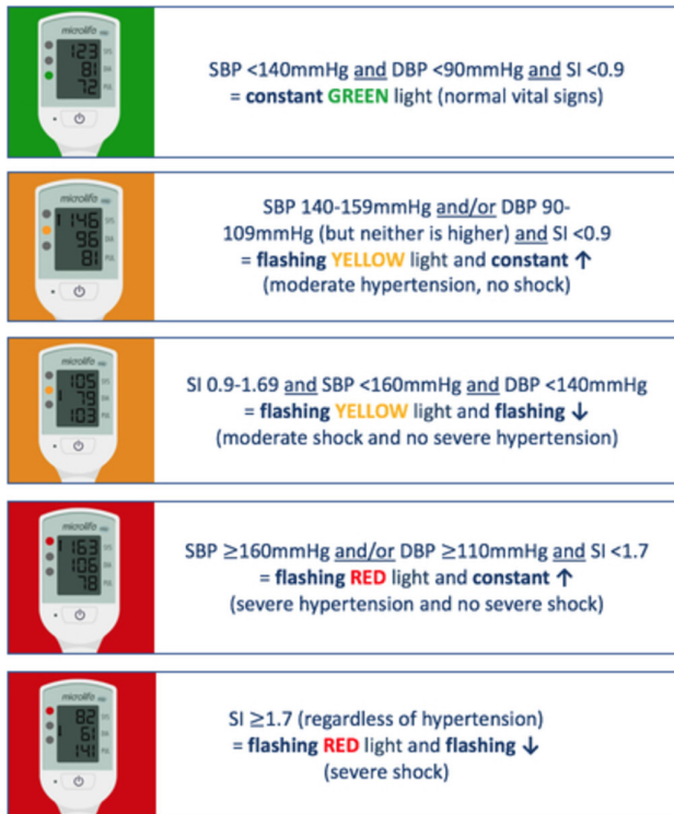
Figure 2 Vital Signs Alert device traffic light early warning system display options. DBP, diastolic blood pressure; SBP, systolic blood pressure; SI, Shock Index.
