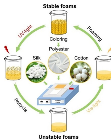
Figure 8. Schematic illustration of a recycled foam coloring process based on photoresponsive foams. Adapted with permission from ref. [141]. Copyright 2019, ScienceDirect, Elsevier B.V.
