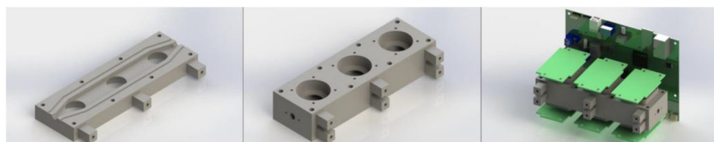
Figure 2. The 6-slotted sensor chamber layout. (left) lower part of the chamber; (middle) assembled chamber; (right) assembled chamber with attached sensors and circuit boards.
