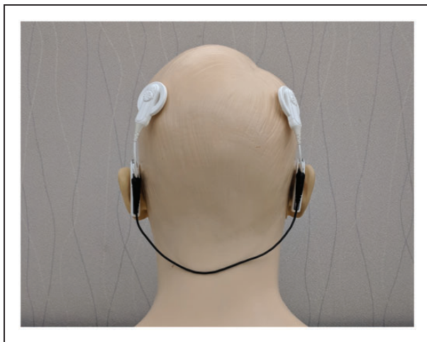
Figure 3. Picture of the wired link. The bidirectional accessory cable was plugged into the right and left accessory ports of the CP810 sound processors.
