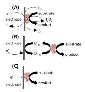
**Figure 3.** The three generations of biosensors showing transition from: (**a**) enzyme dependency to (**b**) mediator use and (**c**) finally to the use of a catalytic electrode.
