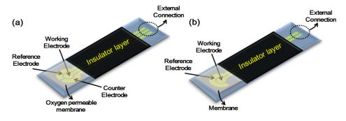
Figure 2. Showing (a) amperometric and (b) potentiometric electrode configurations.
