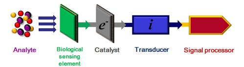
Figure 1. Generalized biosensor schematic showing stages in response to analyte.
