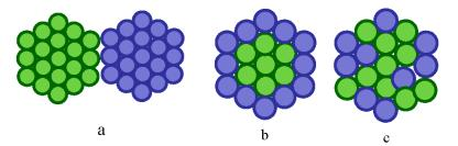
Figure 4. Catalytic structures: (a) heterogeneous, (b) core-shelled and (c) alloyed.
