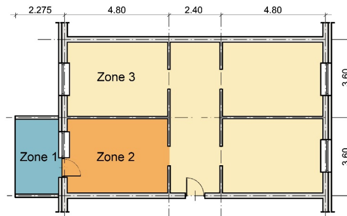
Figure 1. The modelled apartment with thermal zones.
