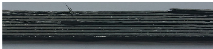
Figure 10. CFRP structure after the tensile test.
